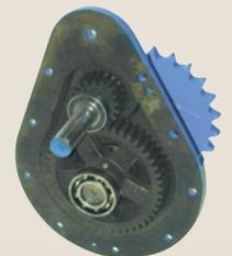
Heavy-duty, cast-iron gathering chain drive gearbox provides rigidity for housing machined gears in the oil-bath transmission (cut-away view).
