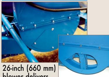
26-inch (660 mm) blower delivers high volumes of silage. Inspection cover removed for easy impeller adjustment (guard removed for viewing).
