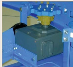
This torque limiter protects the ring and drive gearbox from overload while providing positive drive power (guard removed for viewing).
