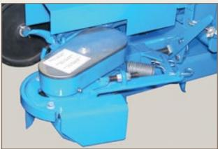
The power cutter's unique design with its spinning action follows the exact curvature of the silo wall.
