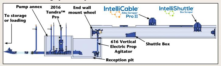
Tundra™ Pro Pump is designed to transfer slurry type manure with limited amounts of sawdust or sand type bedding. The **Tundra™ Pro Pump** can be fed manure via a gutter cleaner or skid steer into a hopper or via a shuttle box located in the cross gutter filling a reception pit.
