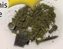
Actual tramp metal removed from magnet.
