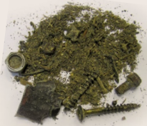
Actual tramp metal removed from magnet.
