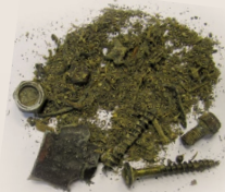
Actual tramp metal removed from magnet.
