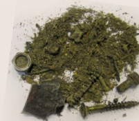
Actual tramp metal removed from magnet.
