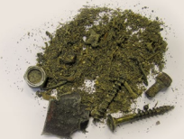
Actual tramp metal removed from magnet.
