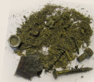
Actual tramp metal removed from magnet.
