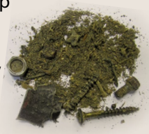
Actual tramp metal removed from magnet.
