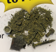
Actual tramp metal removed from magnet.
