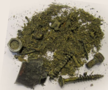
Actual tramp metal removed from magnet.
