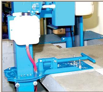
**Foot locking pedal** allows rotation of the agitator to handle many types of slurry waste and improve pit cleanout.
