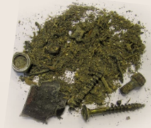
Actual tramp metal removed from magnet.
