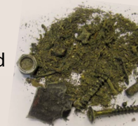
Actual tramp metal removed from magnet.
