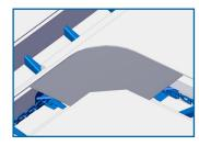
2 Patz Corner Wheels keep the chain on. Large, double-flanged, 12 inch (305 mm) corner wheels are designed to contact only the back of the link. The wheel is through-hardened to a specific hardness that resists wear. Each corner wheel has a greaseable composite bearing.
