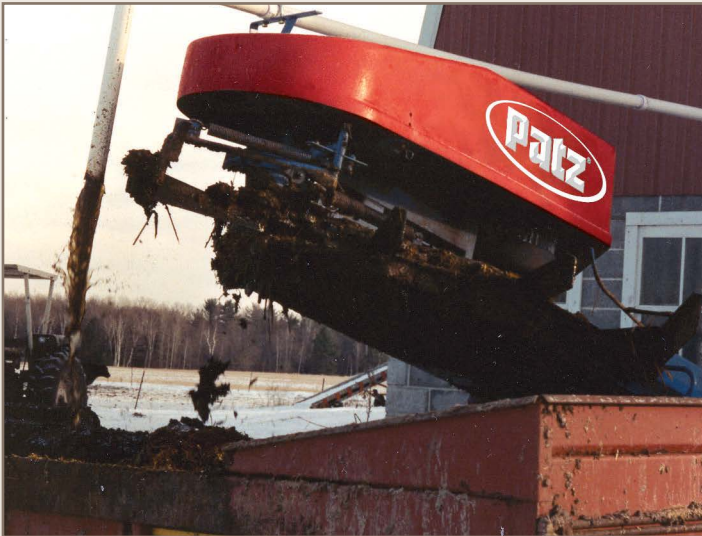
Liquids drop through the screen into the sump. Two screen sizes available: 3/8-inch (9.525 mm) and 5/8-inch (15.875 mm).
