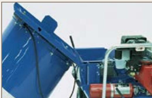
**The deck** is hinged for convenient inspection of the rotor.
