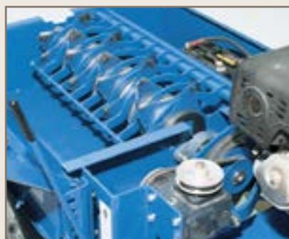
**A single-handle, seven-position grate control** allows varying length of cut and adjusts material flow rate.
