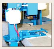
**Foot locking pedal** allows rotation of the agitator to handle many types of slurry waste and improve pit cleanout. **Protection against bearing contamination** with four seals on the lower gearbox output shaft to keep contaminants out.
