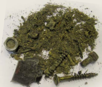
Actual tramp metal removed from magnet.
