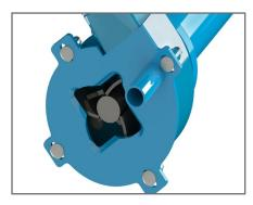
The Shear Plate minimizes clogging. The impeller blades swept-back design increases pumping efficiency. The impeller area is manufactured using heavy, abrasion resistant steel to prevent rust and prolong life.
