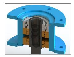
Protection against bearing contamination. The lower bearing's oil-bath chamber has four seals to keep contaminants out.
