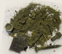
Actual tramp metal removed from magnet.
