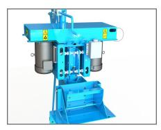
Easy lubrication with convenient oil and grease lines. A transparent oil line makes reading oil levels simple.
