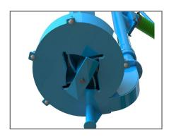
The Shear Plate minimizes clogging. The impeller blades swept-back design increases pumping efficiency. The impeller area is manufactured using AR-400 abrasion resistant steel to prevent rust and prolong life.
