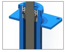
Protection against bearing contamination. The lower bearing's oil-bath chamber has three seals to keep contaminants
