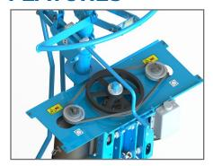
Choose from single motor, 7.5 - 40 HP, or twin motor, 7.5 or 10 HP, speed packages to meet your volume output requirements.
