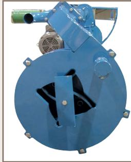
**Easy access to oil reservoir.** End guessing! Inspect oil level conveniently in the semi-transparent oil reservoir at the top of the pump. Patz recommends using an 85W90 oil.
