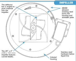
ousing and curved blades are continuously being eeping a constant positive pressure at the discharge point. As the impeller turns, slurry is forced to the outer band area, which becomes larger as slurry approaches the discharge point. More slurry is being constantly added to the impeller blades as slurry moves away.
