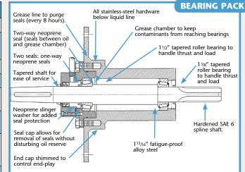
g pack can be entirely removed from the 6"x 6" plined shaft.
