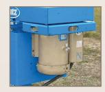
**Unique seal system** extends gearbox bearing life. Gearbox bearing seals can be purged every 8 hours.
