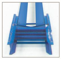
Open pan design provides deep trough for extra capacity and reduces belt friction for lower power requirements. Fin pulley helps avoid material buildup.
