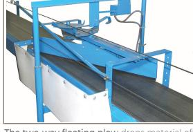
The two-way floating plow drops material off both sides of the conveyor. The belt reverses allowing material to be added at various points. An electrical remote is used to switch between sides. Distribute up to 4 different locations with a 2-motor drive and plow drive assembly. An optional deflector allows for a more accurate drop.
