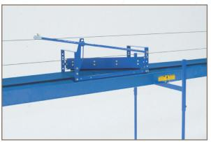
The one-way floating plow drops material off on one-side of the conveyor only. Using a 2-motor drive allows distribution up to two different locations.
