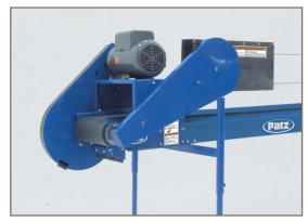
One motor drives both the belt and plow (roller-chain drive) to distribute one location or two different locations. The plow automatically reverses smoothly around a pulley at each end of the conveyor with continuous-loop cable drive.
