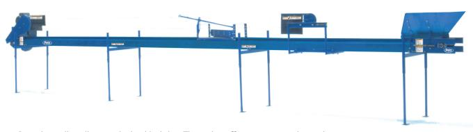
Stands easily adjust to desired height. They also offer support and couple conveyor sections for ease of installation.
