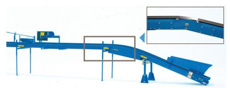
Elevate material and then convey flat with an adjustable elbow. The belt stays concave with a deep trough when passing over the elbow for maximum capacity.
