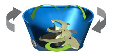
Gray arrows indicate direction of screw rotation. Green arrows indicate Balanced Flow  $^{\text{TM}}$  of feed
