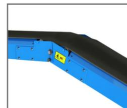
Elevate material and then convey level. When passing the elbow, the belt stays concave with a deep trough for maximum capacity.
