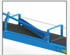
One-way Floating Plow drops feed off one side of feeder only. A 2-motor drive allows different rations to be fed to two lots.
