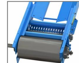
Convenient adjustment for belt tension and tracking. A 5/8" screw provides up to 20" of belt take-up. The pulley is finned for clean-out.
