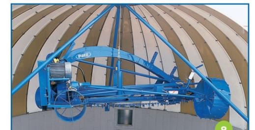
**8** When refilling the silo, the 98C can be raised to the top of the dome above the silo wall providing you with every inch of feed storage.
