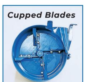
**5** The high-capacity blower's high-strength, corrosion-resistant steel impeller blades with welded studs are adjustable to allow close tolerance for maximum blower efficiency and longer service life. Choose from flat or cupped blades.
