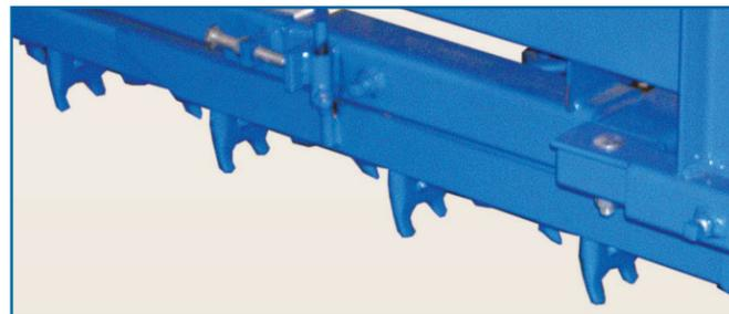
Easy setscrew adjustment of chain tension!
