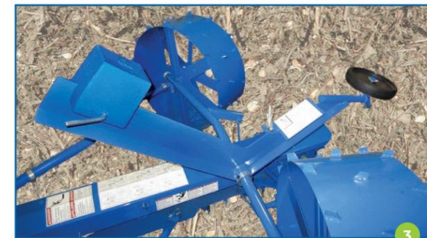
**3** The 98C's dept-of-cut control and counterweight for the gathering chain eliminate daily adjustments while providing a full flow of silage every feeding — right to the bottom of the silo.
