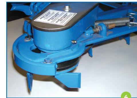
**4** The power cutter's unique design with its spinning action follows the exact curvature of the silo wall. Spring tensions keep the spinning, self-sharpening knives in position resulting in a "clean-shaven" silo wall. An oil-bath for the roller chain-driven power cutter provides long service life. Wear shoe is easy to replace and keeps maintenance economical. (Guard removed for viewing.)
