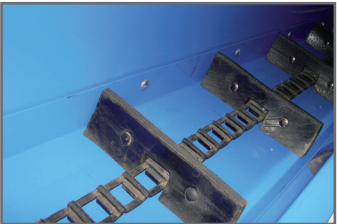
Detachable Steel Chain with steel-braced, 2 ½" high rubber flites and 12" spacing delivers high capacity.
