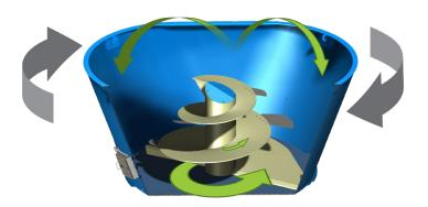
Gray arrows indicate direction of screw rotation. Green arrows indicate Balanced Flow  $^{\text{TM}}$  of feed
