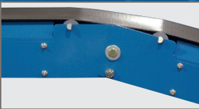
Elevate 0° - 30° and then Convey Level with an adjustable decline — Belt stays concave when passing over the elbow for maximum capacity
