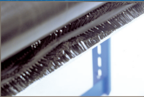
An Optional Wiper or powered brush (shown) belt wiper cleans the top surface of non-cleated belting
