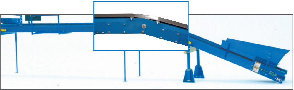
Elevate Material and then Convey Level with an adjustable elbow. The belt stays concave with a deep trough when passing over the elbow for maximum capacity (shown with optional end hopper).
